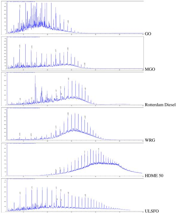
Figure 1: GC-FID chromatograms of the six tested fuel oils
