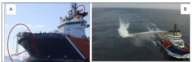
Figure 2:A: Response systems installed on MS Strilborg (low-dosage dispersant<br/>application followed by artificial turbulence using high-capacity water<br/>flushing bow booms<br/>B: Mechanical dispersion using Fi-Fi monitors on thin oil films
