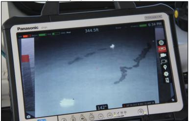
Figure 2 – shows the viewing screen, on the bridge of the Earl 2 vessel, illustrating the outputs of the Infra-Red sensor. The image shows two vessels and two lines of oil in the water (as the oil was released from the vessels).
