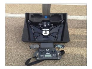
Figure 3 - UAS and Mobile Control Station (MCS) provided by Sky Futures – the MCS screen on the controls allows you to see what the UAS camera is filming
