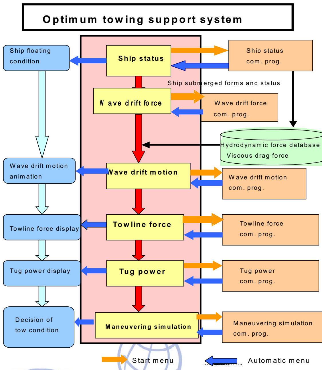
Figure 12 Flow of Optimum Towing Support System
