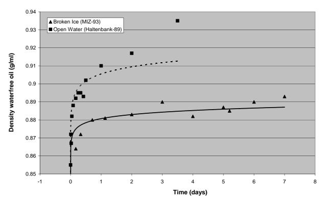
*Figure: 5: Density (g/ml) of the crude oil as a function of time for both the Haltenbank-89 and the Marginal Ice Zone 1993 experiment*
