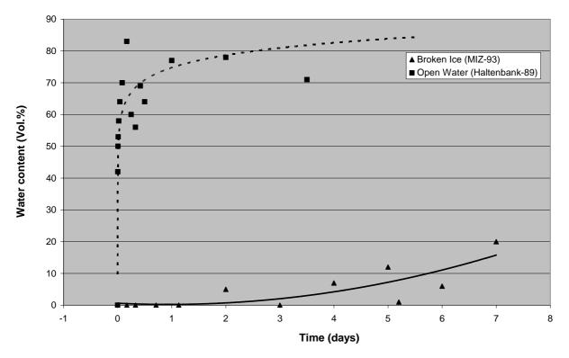
Figure 6: Water uptake (volume %) of the crude oil as a function of time for both the Haltenbank-89 and the Marginal Ice Zone 1993 experiment
