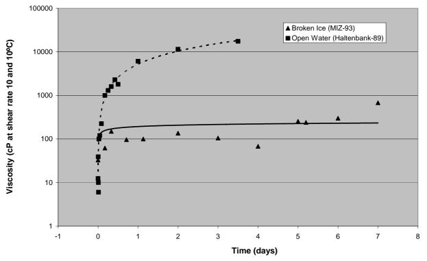
*Figure 7:* Viscosity of emulsion (cP, shear rate 100 or 10 at 10°C) of the crude oil as a function of time for both the Haltenbank-89 and the Marginal Ice Zone 1993 experiment
