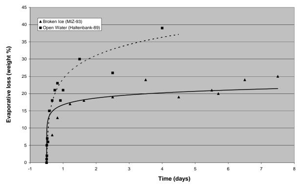
Figure 4: Evaporative loss (weight %) of the crude oil as a function of time for both the Haltenbank-89 and the Marginal Ice Zone 1993 experiment
