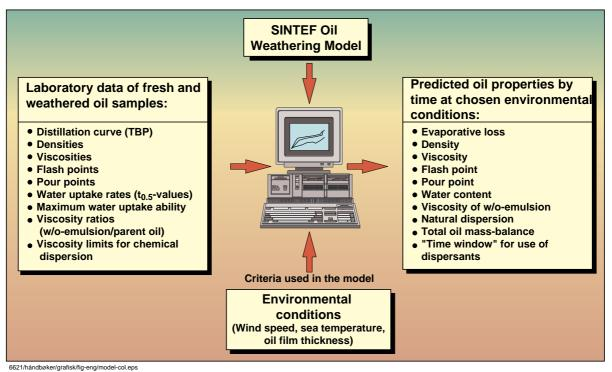
Figure 1: SINTEF Oil Weathering Model.
