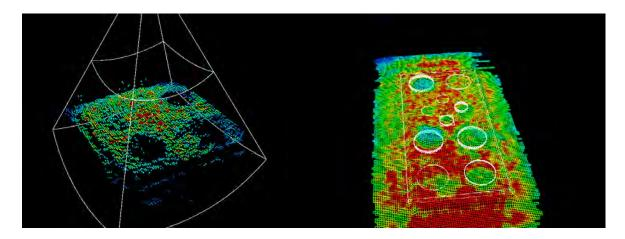
Figure 12: Typical snapshot obtained with Echoscope 3D-Camera (left); averaged reflectivity measurement over the targets (right; note the difference between the nominal and the actual location of some oil patches)
