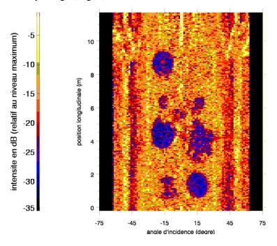
Figure 6. Echo intensity level obtained with the Seabat 8101 multibeam echosounder operated along a line exactly in the middle of the sand tank.
