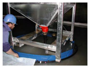
Figure 2: (left) The ten patches on the sand floor, before oil filling and water flooding. (right) Filling of an oil patch.
