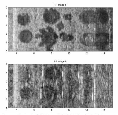
Figure 5: Sonar image obtained with Edgetech DF-1000 at 400 kHz (upper) and 100 kHz (lower.
