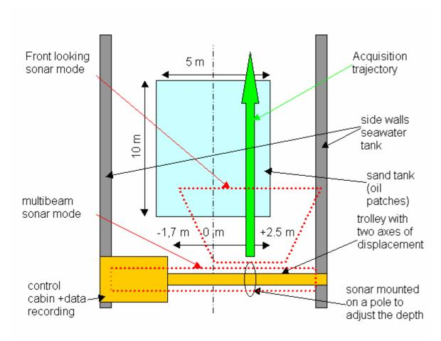
Figure 3: Sketch of the sonar deployment geometry over the sand tank
