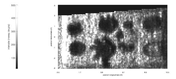
Figure 4: Reflectivity map obtained with sidescan sonar Klein 5500
