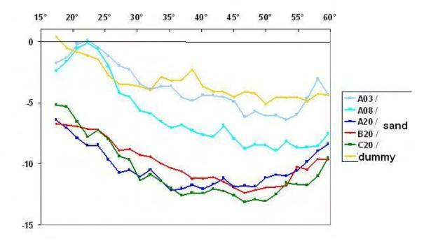
Figure 11: Backscattering strength contrast (referenced to the sand response) of the various oil patches as a function of incident angle, measured by the front-looking multibeam interferometric system COSMOS. (cf fig.1 for the meaning of A03...C20)
