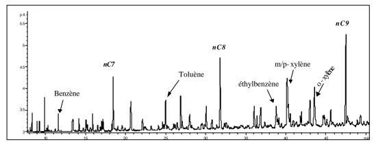
Figure 6: GC chromatogram of the C9 fraction of the Prestige fuel oil n°6.
