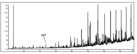
Figure 5: GC chromatogram of the  $C_{20}^{-1}$  fraction of the Prestige fuel oil n°6.
