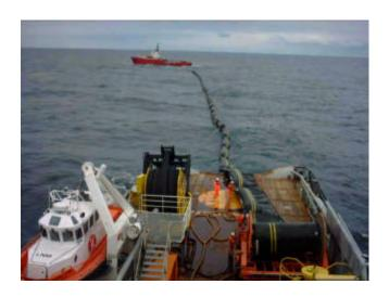
Figure 7: Deploying the boom
