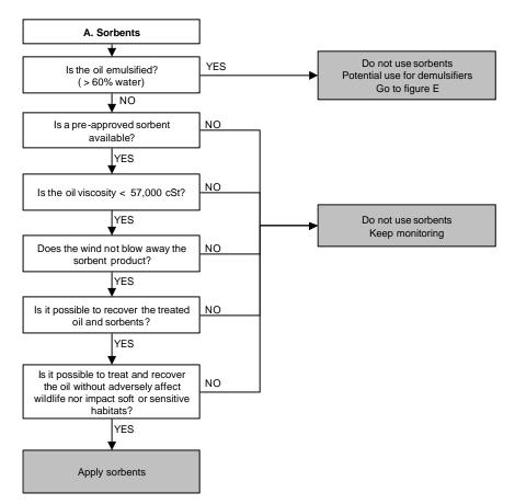
Figure 10 Decision tree to determine if synthetic sorbents can be used
