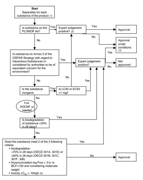
Figure 2 Pre-screening scheme for the assessment of oil spill chemicals, based on OSPAR Recommendation 2000/4 on a Harmonised Pre-screening scheme for Offshore Chemicals
