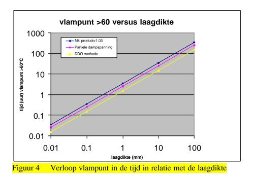
The figure shows that all three methods show a clear relationship with the layer thickness, but that with the DDO-method the flashpoint criterion is met faster then with the other methods. For oil spill recovery the area between layer thickness of 0,1 to 1 mm is most important. At a layer thickness of 0,1 mm flashpoint will exceed 60 °C within the hour, whereas it will take several hours when dealing with a layer of 1 mm thick.
