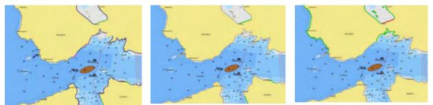
Figure 5 Example of application of the model for prioritization. To the left, the shoreline is classified according to shoreline type. The middle figure shows the results when initial sensitivity is included. The figure to the right shows the results when overlap with high priority environmental resources is included in the evaluation
