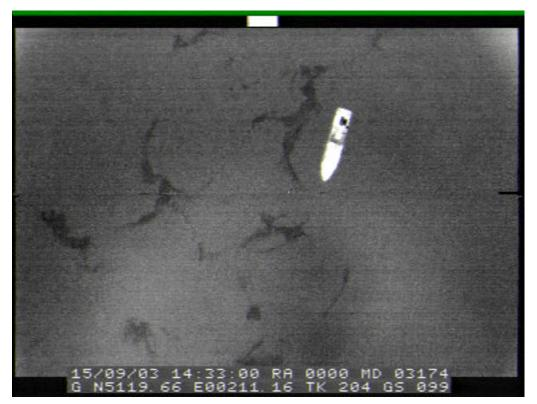
Figure 2: Infra Red (IR) sensor image of 'Tricolor' oil pollution observed on 15.09.03 (time in UTC), with w/o emulsions clearly visible as black patches, with the IR sensor in 'white hot' mode (photo MUMM).
