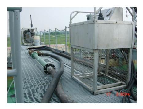
Figure 9. In line mixer on deck connected to discharge hose just before recovery tanks.
