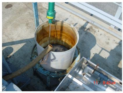
Figure 4. Mixing tank for decanted water sampling.
