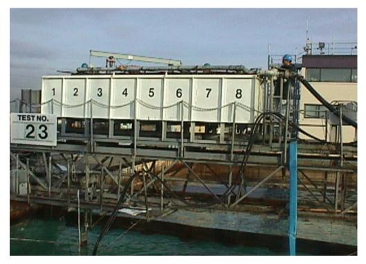
Figure 3. Recovery tank on auxiliary bridge.
