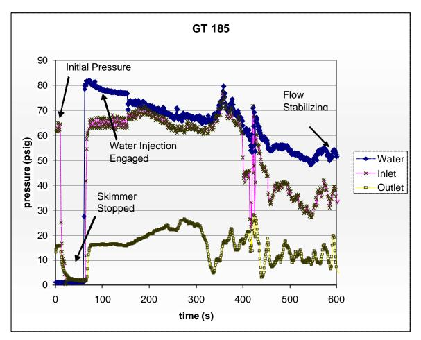
Figure 3 Testing Bitumen with Annular Ring 10.2 cm (4")
