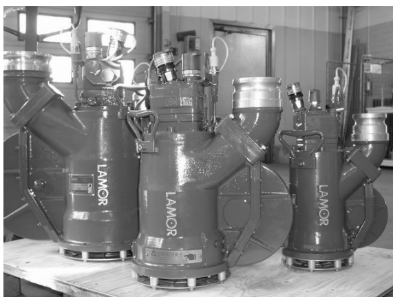
Figure 7 The Lamor GT-A Pump Series with a Cutaway Pump to the right
