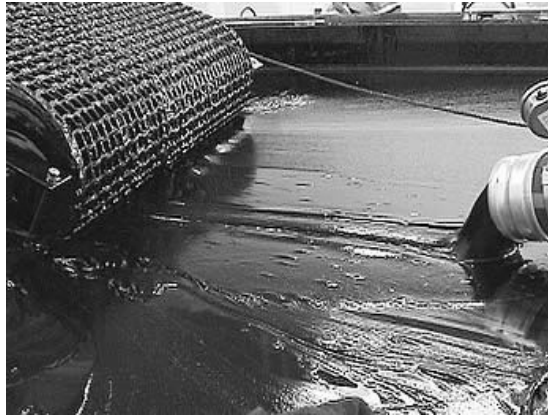
Figure 11 ERE Skimmer and Discharge from TSD 150 Pump
