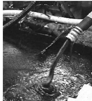
Figure 10 GT-185 w. Inlet/Outlet Steam Injection and Discharge from Test
