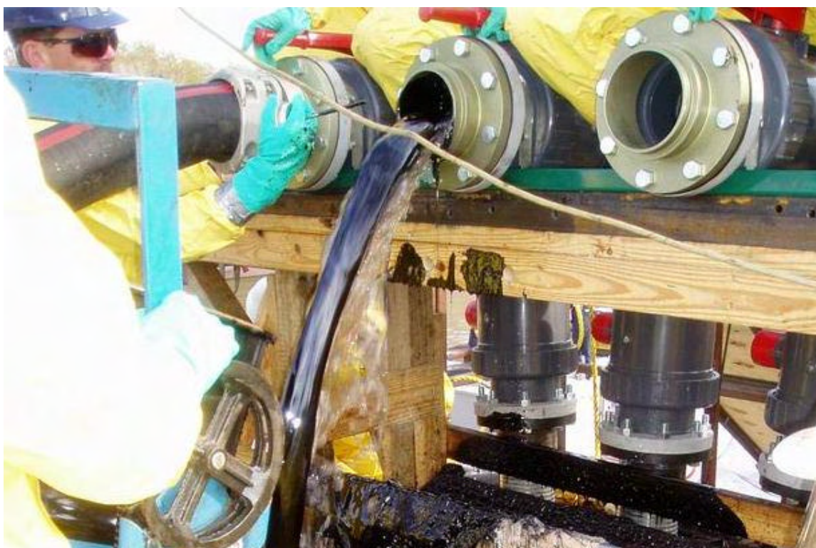
Figure 13 Discharge of 410,000 cSt oil and lube water in 150 m test with GT-185
