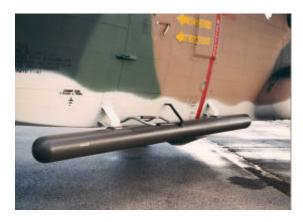
Figure 3 An Ericsson SLAR antenna on one of the CASA 212 aircraft that are operated by the Portuguese Air Force for fishery protection.
