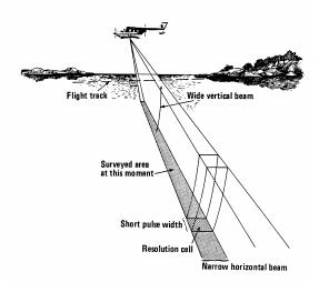
Figure 3 The basic principle of the Side-Looking Airborne Radar (SLAR).
