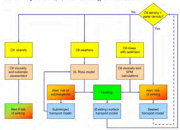
General approach to modelling oil sinking or submerging. Traffic light – Red, Amber, Green shaded boxes indicate probability of submergence or sinking.
