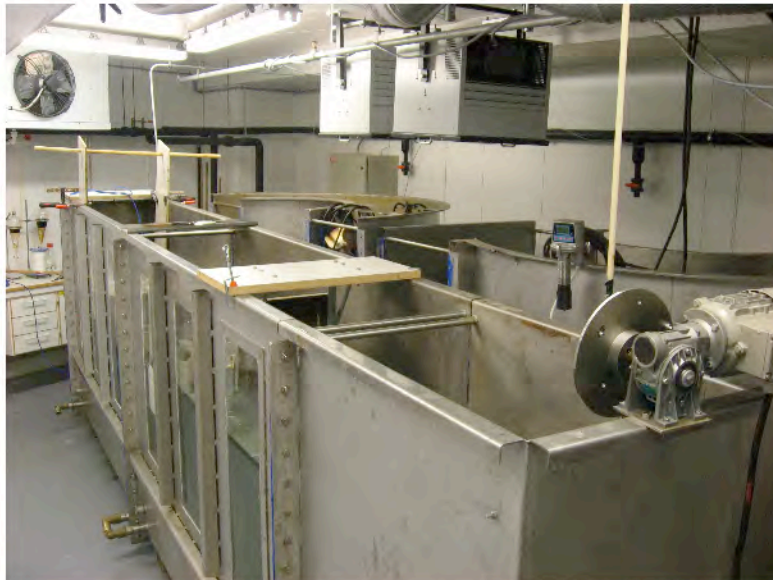
Figure 2. Sketch and photograph of the setup for the breaking wave experiments. In the photograph, the semi-circular ends of the flume in its elliptical configuration can be seen to the right of the straight flume section in the foreground.
