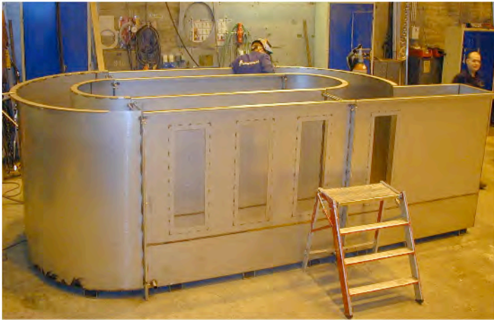
Figure 1 Meso-scale flume at SINTEF for long-term weathering studies of oils and petroleum products.
