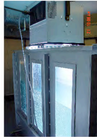
Figure 1 Meso-scale flume at SINTEF for long-term weathering studies of oils and petroleum products.
