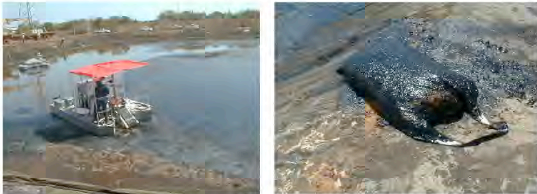
Figure 3 – Recovery of Heavy Oil with Mechanical Feeder Skimmer (lhs) and Disposable Bag Containing Recovered Heavy Oil (rhs)
