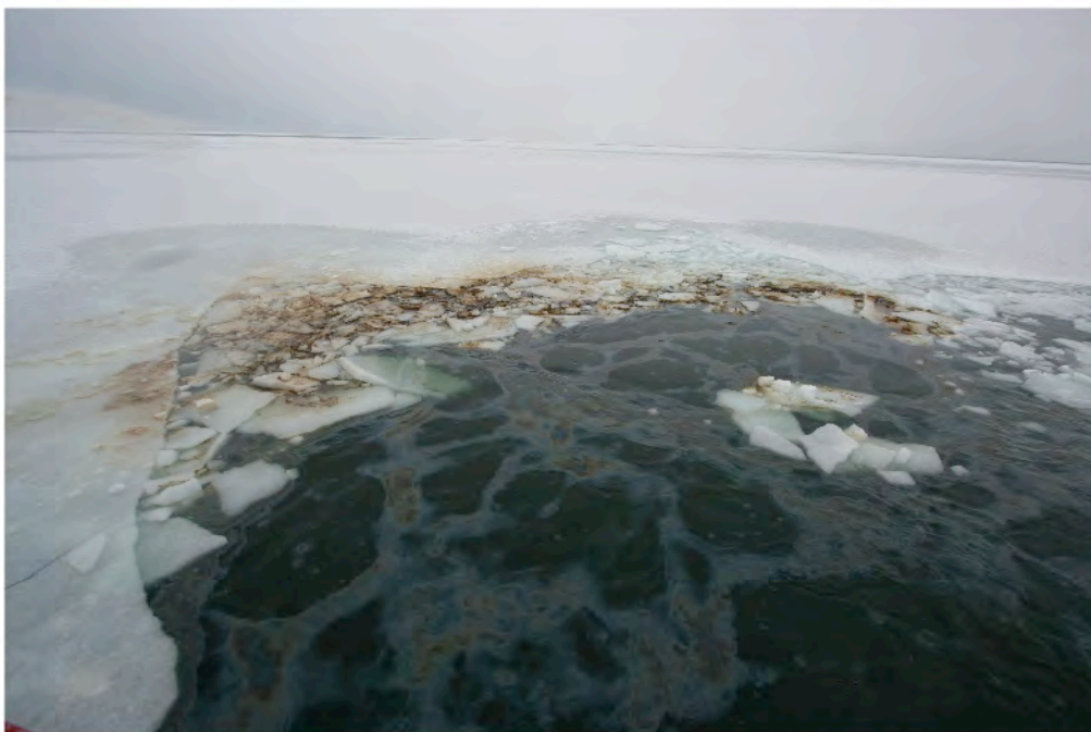
Figure 2: Visual observation of the resurfaced oil after two stages of oil dispersion in Test 3, where the first stage of cleaning effort was made by providing mixing energy only without mineral fines.
