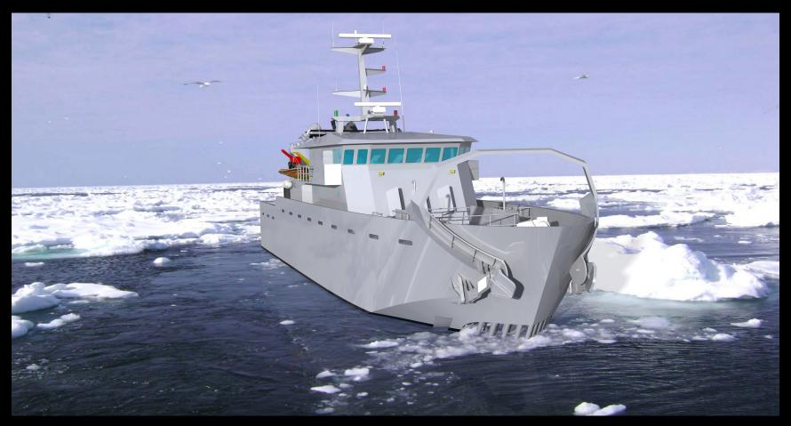
A harrow is incorporated into the bow in order to push aside large blocks of ice
