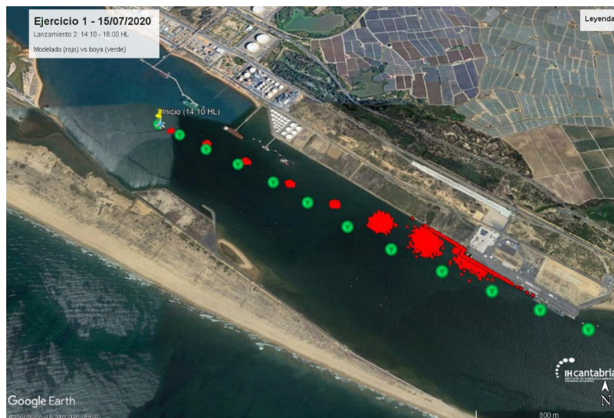
Figure 2. Validation of the system with drifters in the Huelva Estuary. Red: model simulation, Green: drifter trajectory.
