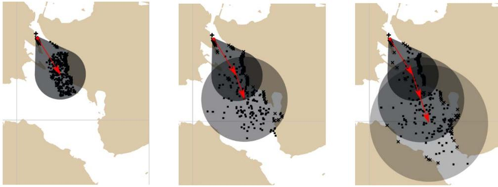
Figure 7. Comparison of oil drift calculation models and Fays' spreading tables (Case 2. Collision of a cargo ship near Savonlinna) [Map: © National land survey of Finland 2018]
