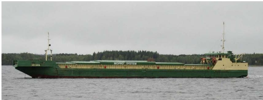
Figure 1. Saimax-class cargo vessel (L82 m x B12 m x D4.2 m, NT 2500 t)
