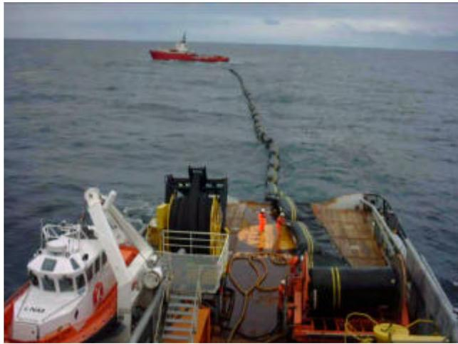
Figure 7: Deploying the boom
