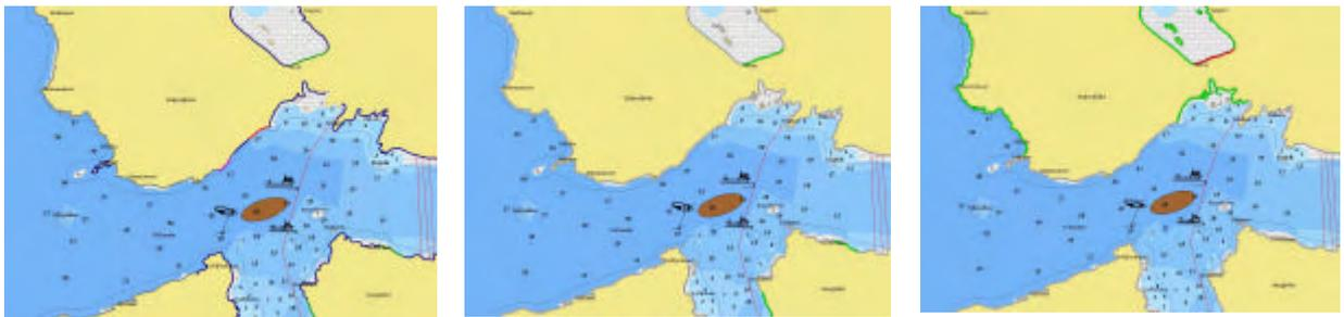
Figure 5 Example of application of the model for prioritization. To the left, the shoreline is classified according to shoreline type. The middle figure shows the results when initial sensitivity is included. The figure to the right shows the results when overlap with high priority environmental resources is included in the evaluation
