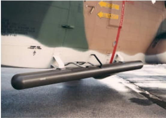
**Figure 3** An Ericsson SLAR antenna on one of the CASA 212 aircraft that are operated by the Portuguese Air Force for fishery protection.
