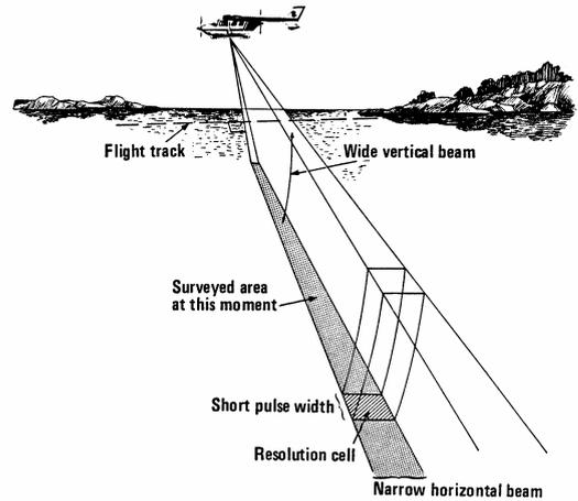
**Figure 3** The basic principle of the Side-Looking Airborne Radar (SLAR).
